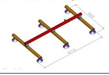
• Put the Jig on the panel and make sure the suction cup could sucks the panel.
